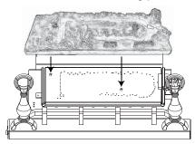
4.2.1 Place the fibre burner cover onto the two locating studs screwed into the pan burner.
